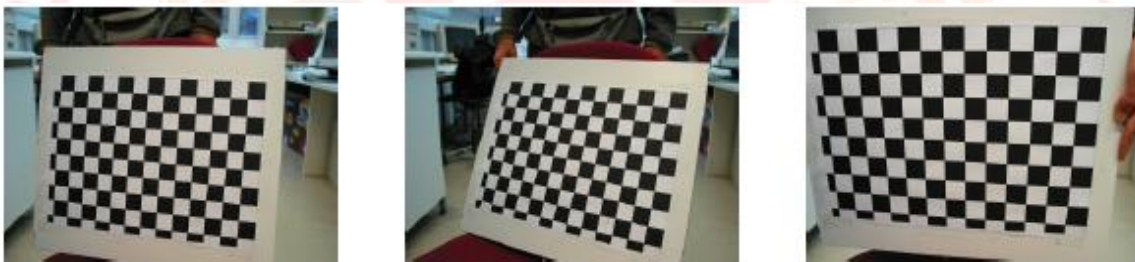
Figure 2: For calibrating our camera we capture images of a chess pattern at random positions and orientations
